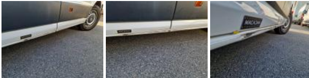
Sliding door R, Dent(s), Repair and paint (complete)
