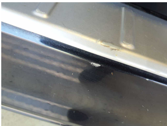
Damage 12: Rear bumper: Rear bumper - Scratch(es) - Paint
