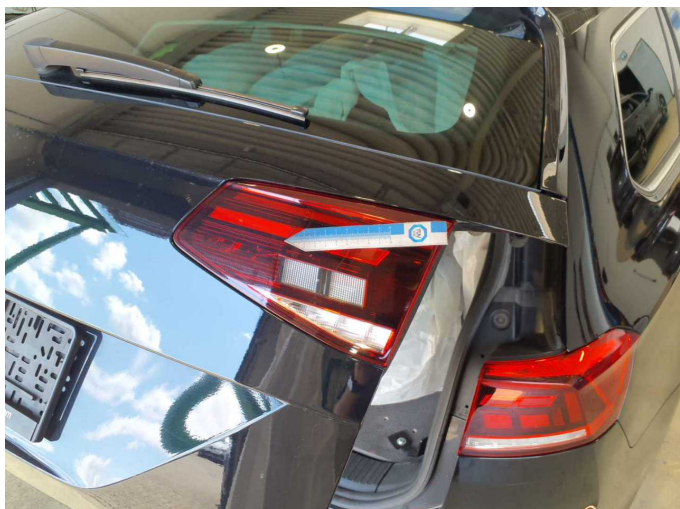
Damage 10: Tail light: Tail lamp - right side - Broken / torn - Replace
