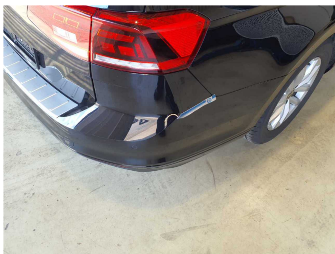
Damage 12: Rear bumper: Rear bumper - Scratch(es) - Paint
