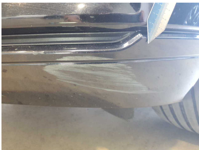
Damage 13: Front bumper: Front bumper - Scratch(es) - Paint
