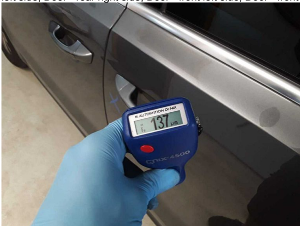
Repainting 1: Sill - left side, Side panel - rear right side, Door - re... left side, Door - rear right side, Door - front left side, Door - front
