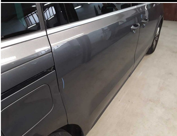
Damage #6: Sliding door, right: Sliding door with glass panel - Scratched - Smart repair
