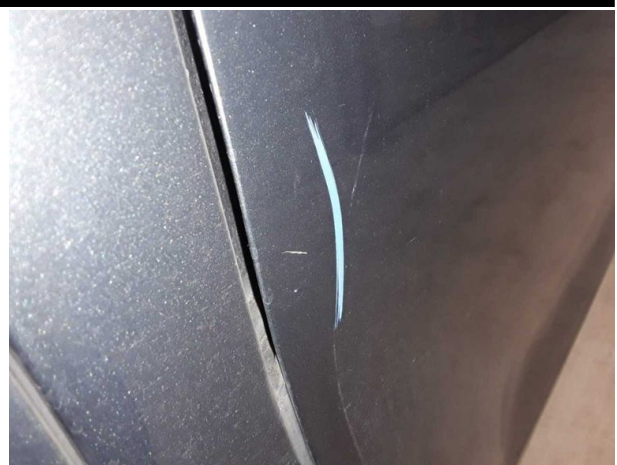
Damage #6: Sliding door, right: Sliding door with glass panel - Scratched - Smart repair
