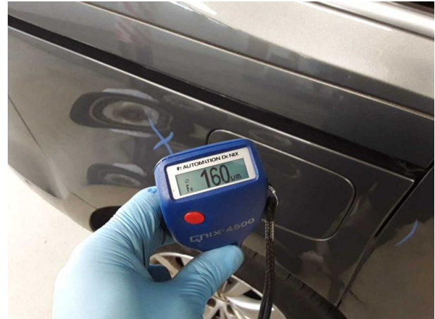
Repainting 1: Sill - left side, Side panel - rear right side, Door - re... rear left side, Door - rear right side, Door - front left side, Door -
