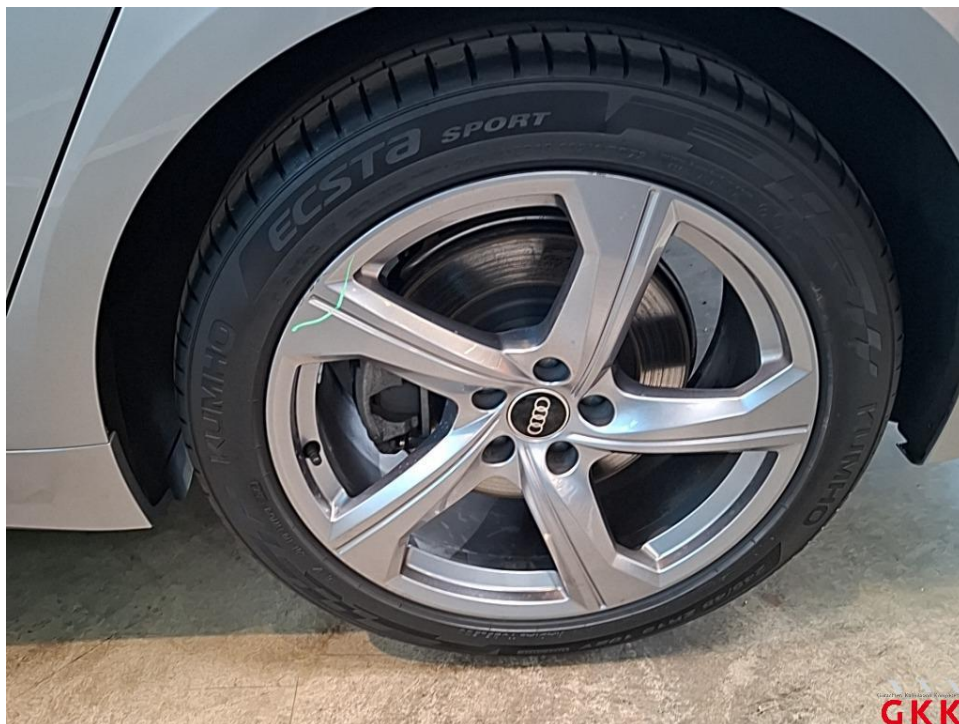
Picture 19 LM wheel, rear left, scratched, depreciation
