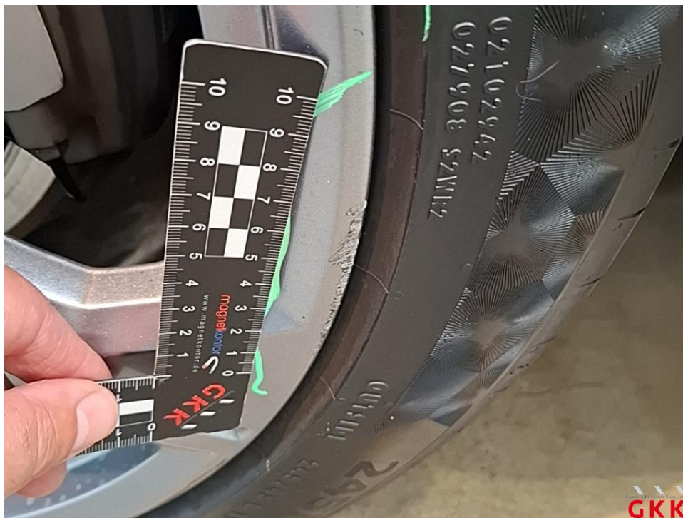
Picture 22 LM wheel, front left, scratched, depreciation
