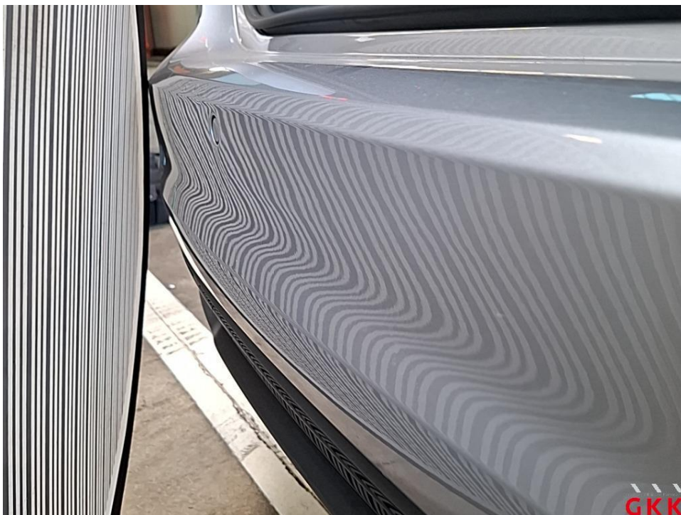
Picture 17 bumper rear, panel -painted-, deformed, replace
