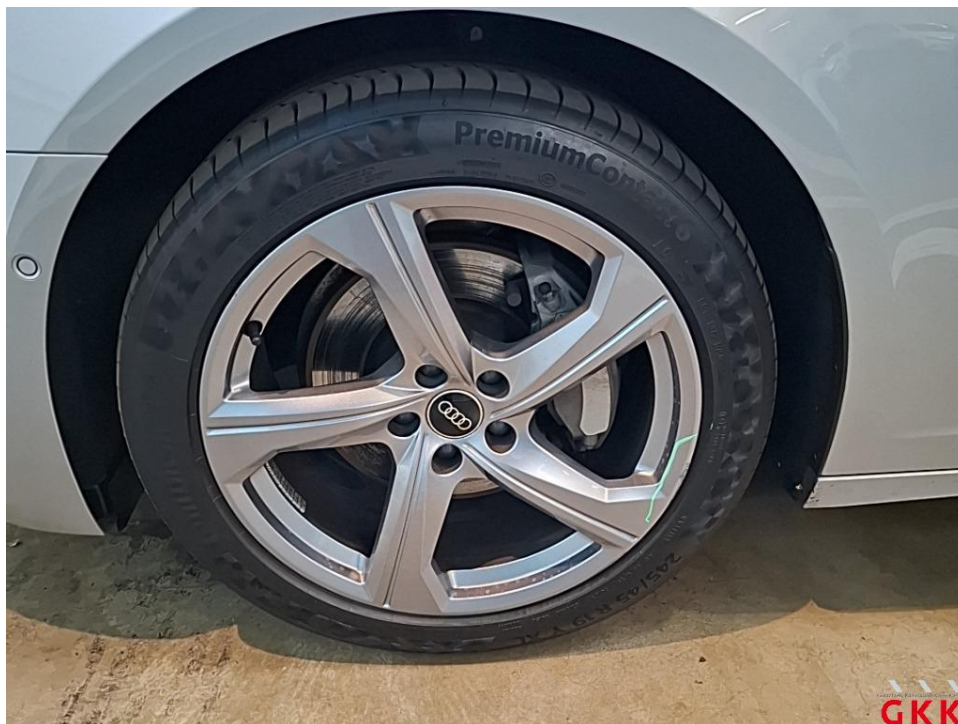
Picture 21 LM wheel, front left, scratched, depreciation
