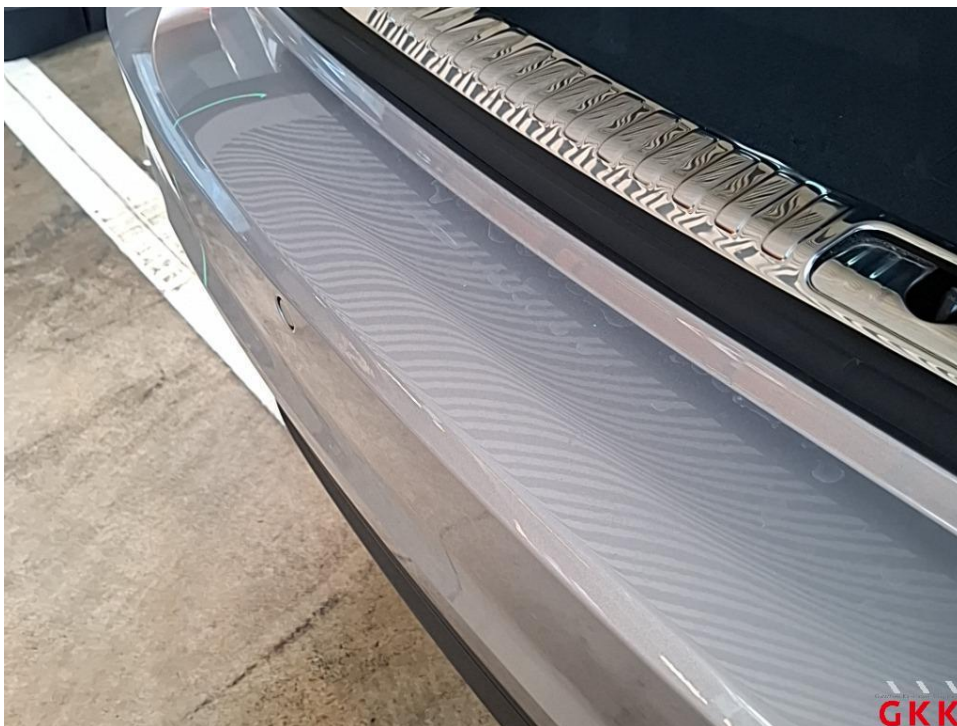
Picture 18 bumper rear, panel -painted-, deformed, replace
