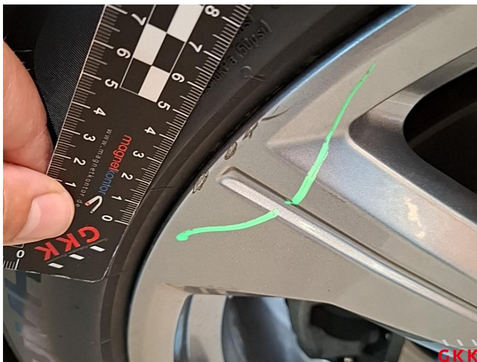
Picture 20 LM wheel, rear left, scratched, depreciation
