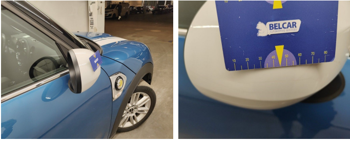
Side View Mirror Right // Painting-scratch
