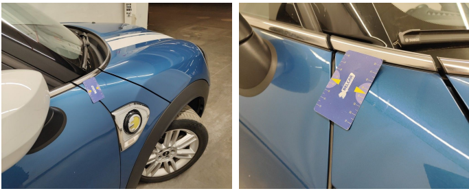
Wing Front right // Polish-scratch
