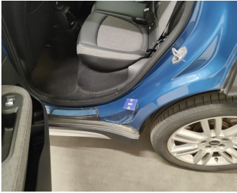
Rocker Panel Left // Polish-scratch
