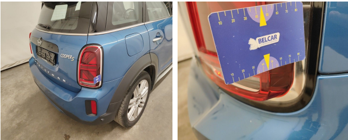
Light / Rear Right / Replace-scratch
