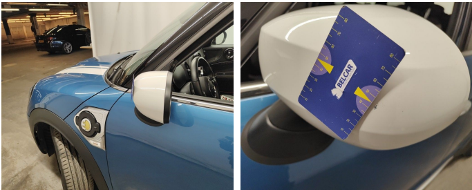
Side View Mirror Left // Painting-scratch
