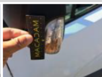
Mirror side repeater L, Broken, Replace
