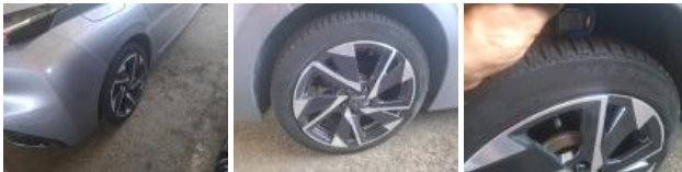
Tyre FR, Out of tolerance, Replace
