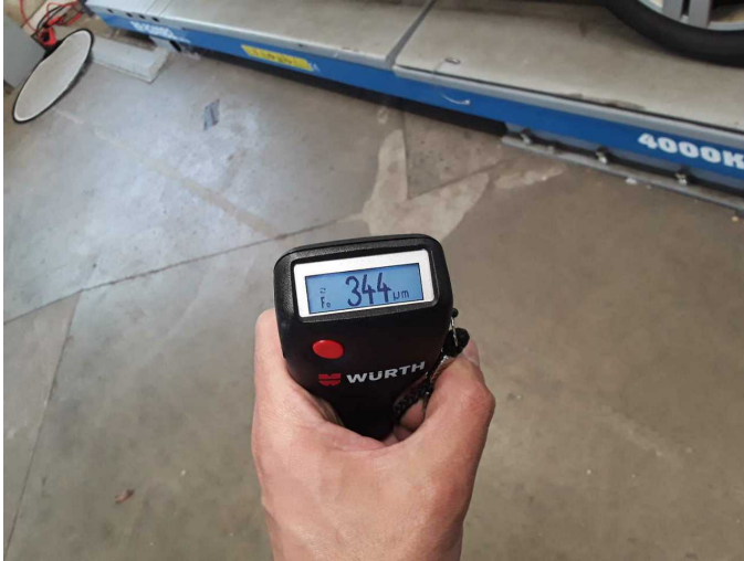
Repainting 1: Side panel - rear left side, Side panel - rear right side, Door - front right side
