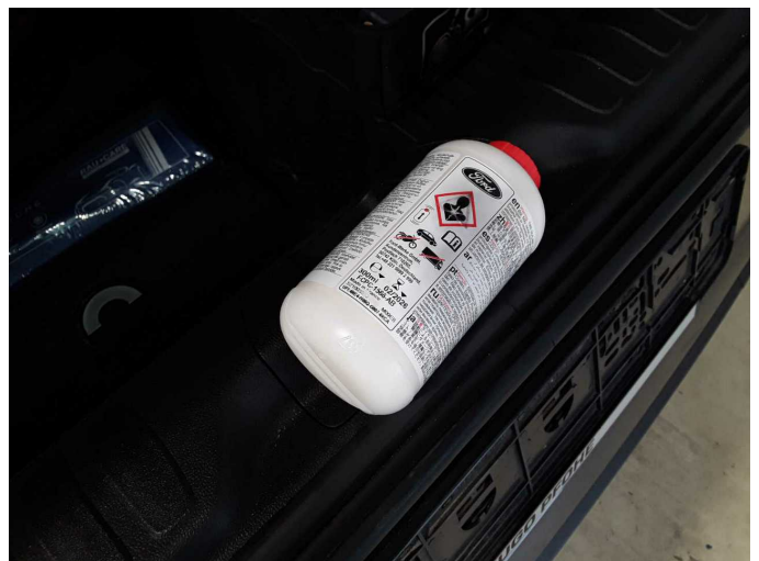
Damage 3: Equipment: Tirefit filler - Expired - Replace
