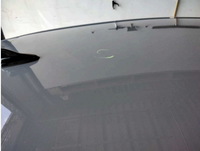
Damage 3: Roof: Roof - dent(s) - Smooth repair work
