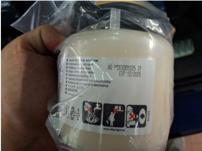
Damage 1: Equipment: Tirefit filler - Due - Replace
