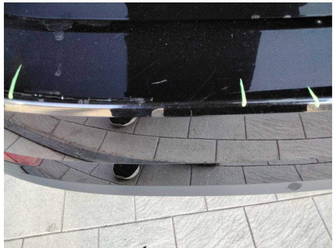
Damage 5: Rear bumper: Rear bumper - Scratch(es) - Paint
