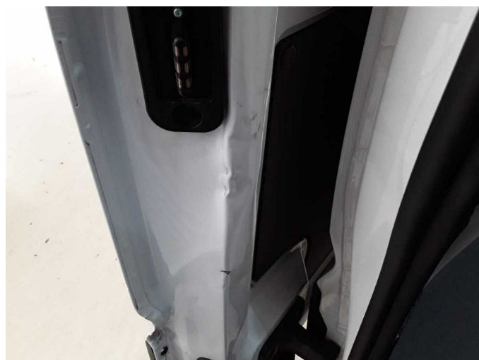
Damage 7: Sliding door, right: Sliding door (innen stark verformt) - Unprofessionally repaired - repair according to calculation
