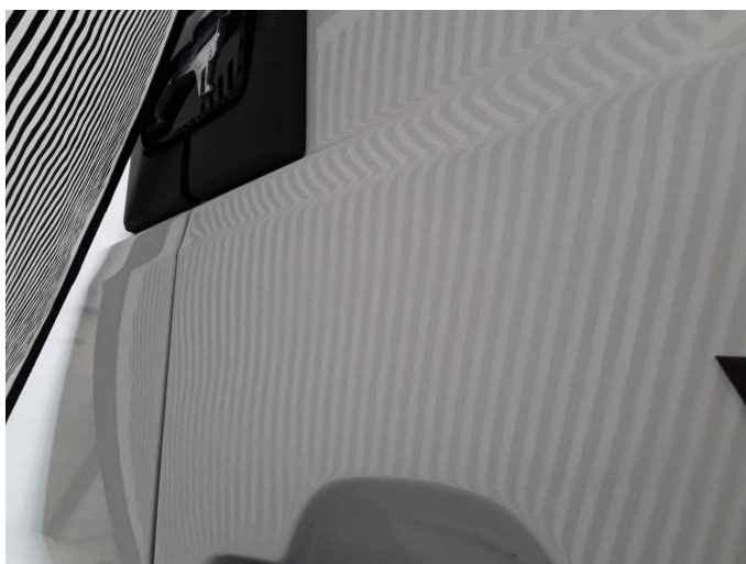
Damage 5: Boot lid / rear door: Rear door - right side (Schleifspuren sichtbar) - Unprofessionally repaired - Paint
