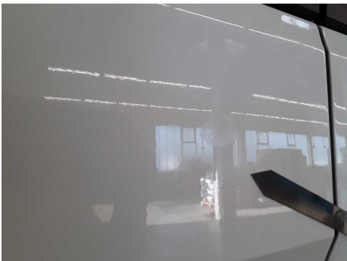
Damage 4: Boot lid / rear door: Rear door - left side (Schleifspuren sichtbar) - Unprofessionally repaired - Repair and paint
