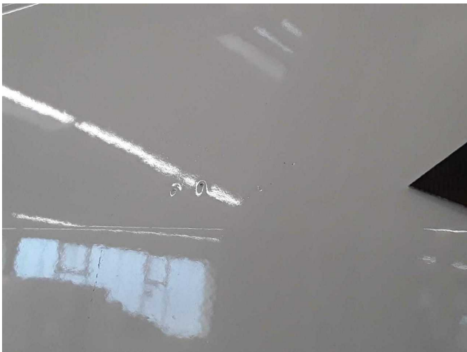
Damage 6: Side panel - rear right side: Side panel - Unprofessionally repaired - repair according to calculation
