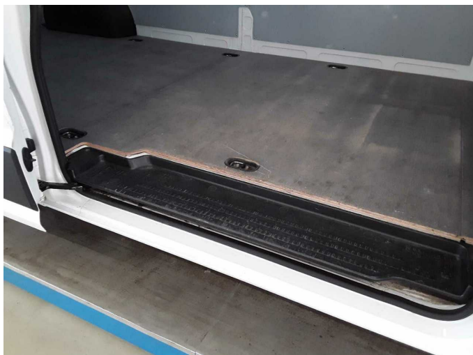
Damage 2: Rear of vehicle: Wooden floor - Scratched - Loss in value
