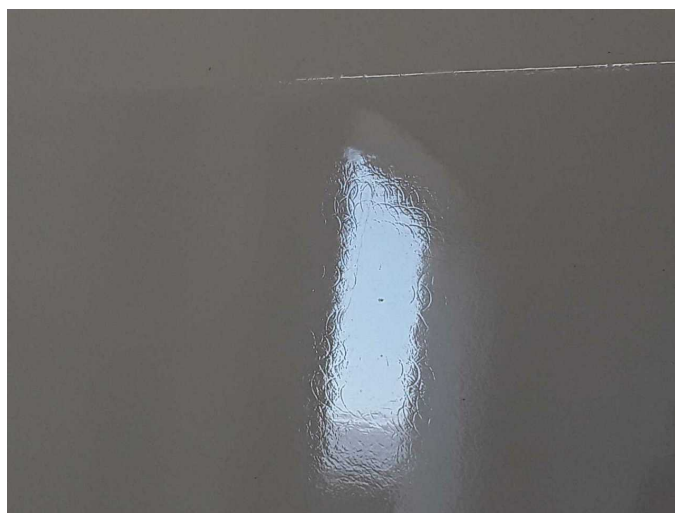
Damage 5: Boot lid / rear door: Rear door - right side (Schleifspuren sichtbar) - Unprofessionally repaired - Paint
