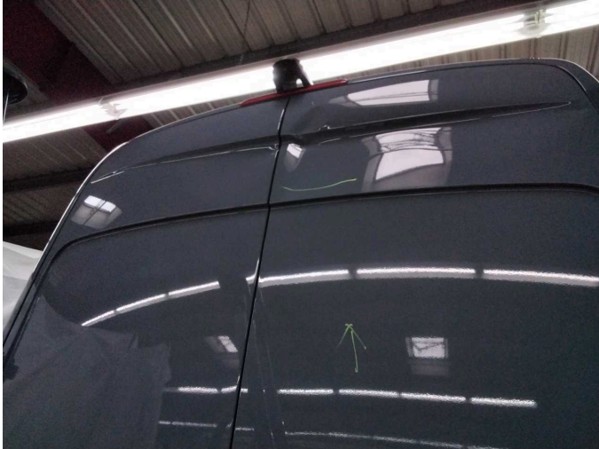
Damage 3: Boot lid / rear door: Rear door - right side (Teillackierung) - Dent / paintcoat damage - Repair and paint
