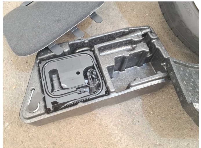
Missing part 1: Equipment: Tirefit filler - Missing - Replace
