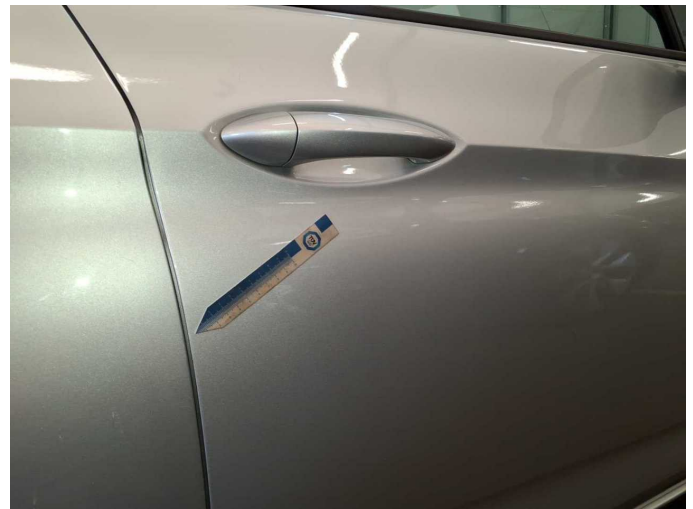
Wear and tear 7: Door - front right side: Door - Scratch(es) - No deduction
