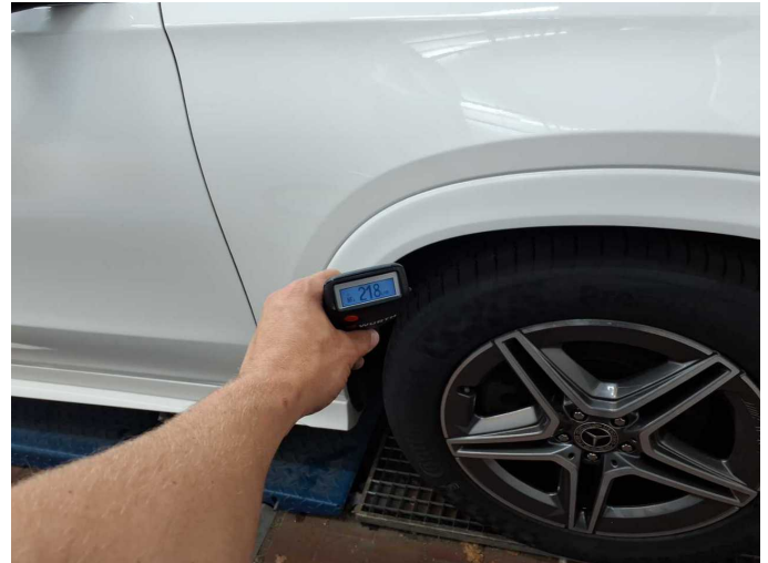
Repainting 1: Mudguard - right side, Side panel - rear right side, Door - rear right side, Door - front right side
