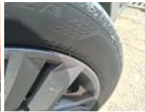
Tyre FR, Out of tolerance, Replace
