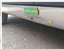
Bumper R, Scratch(es), Repair and paint (complete)
