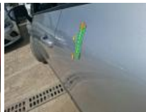
Door RL, Dent(s), Repair and paint (complete)
