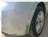
Bumper R, Scratch(es), Repair and paint (complete)
