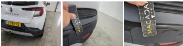
Bumper corner RL, Stone chip(s), Repair and paint (complete)
