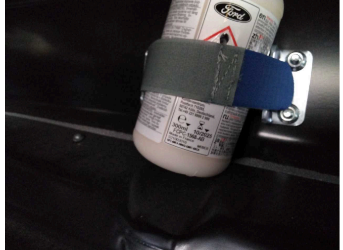
Damage 1: Equipment: Tirefit filler - Expired - Replace
