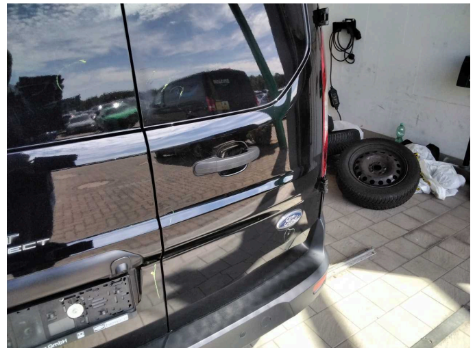
Damage 6: Boot lid / rear door: Rear door - right side - Dent / paintcoat damage - Repair and paint
