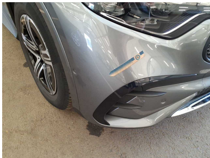
Damage 5: Front bumper: Front bumper - Scratch(es) - Paint
