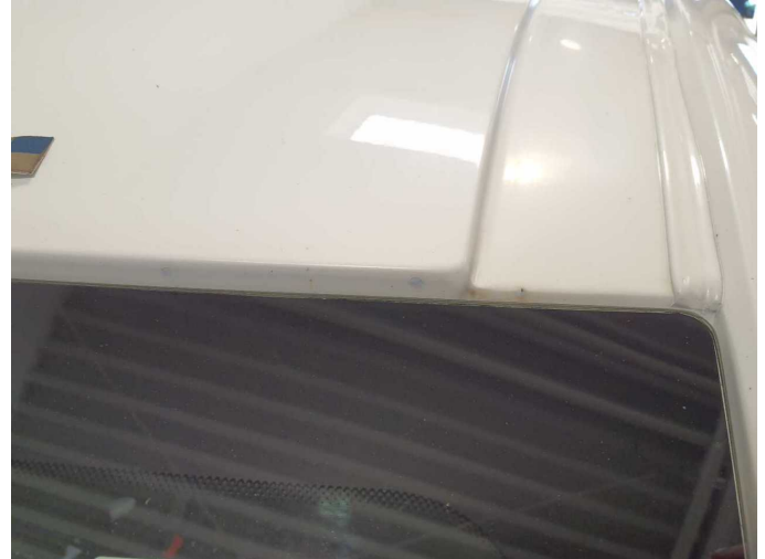
Damage 12: Roof: Roof (Korrosionsbildung) - Scratched - Paint
