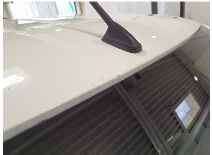
Damage 12: Roof: Roof (Korrosionsbildung) - Scratched - Paint
