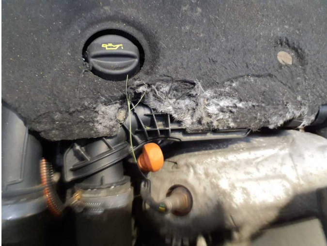
Damage 7: Engine: Engine cover (Mehrkosten möglich) - Damage caused by marten / rodent - Replace
