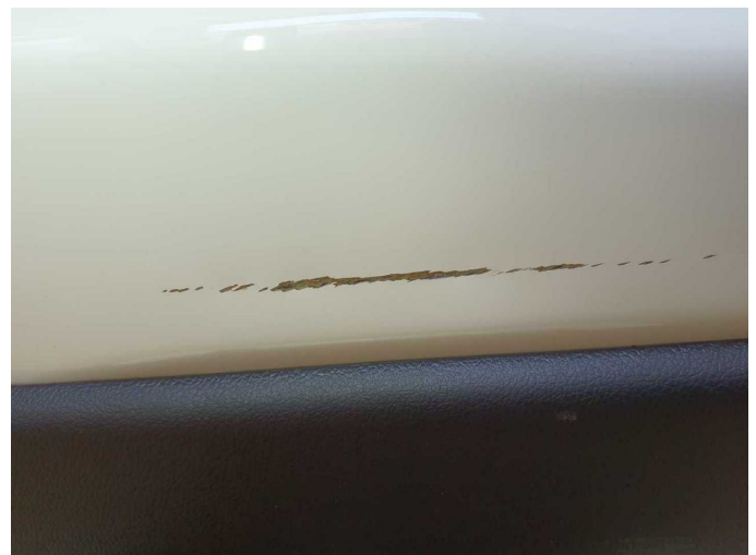
Damage 11: Boot lid / rear door: Boot lid - Corrosion - Repair and paint
