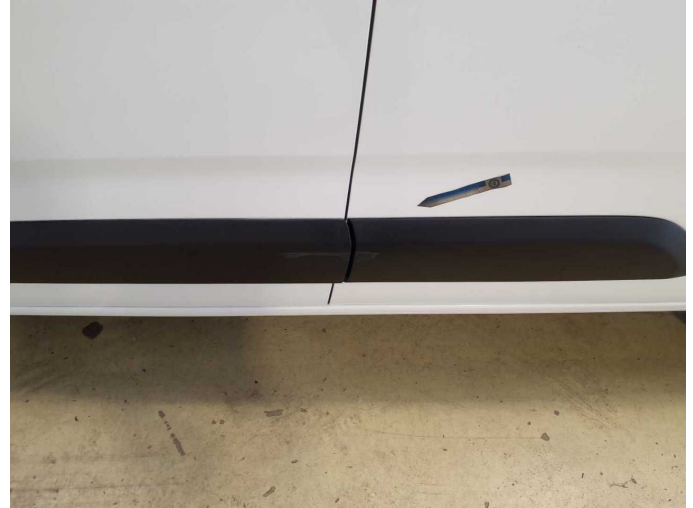
Damage 8: Door - rear left side: Brightware - lower - Scratch(es) - Replace
