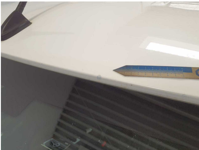
Damage 12: Roof: Roof (Korrosionsbildung) - Scratched - Paint
