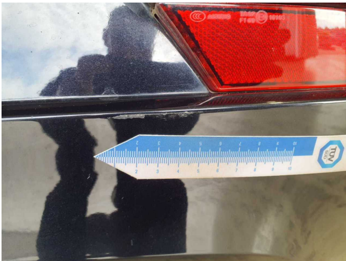
Damage 14: Rear bumper: Rear bumper - Scratched - Paint
