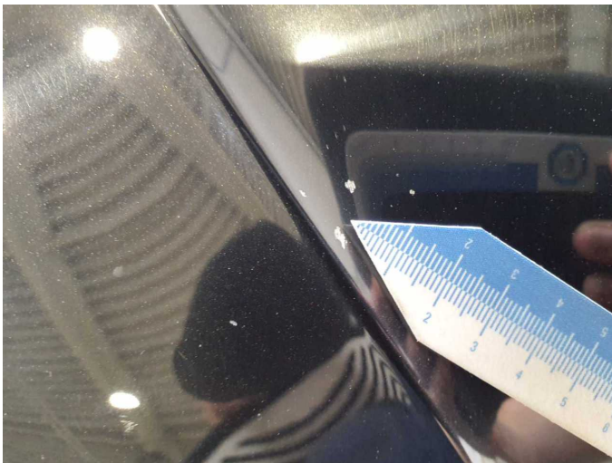
Damage 12: Bonnet: Bonnet - Stone chips - Paint
