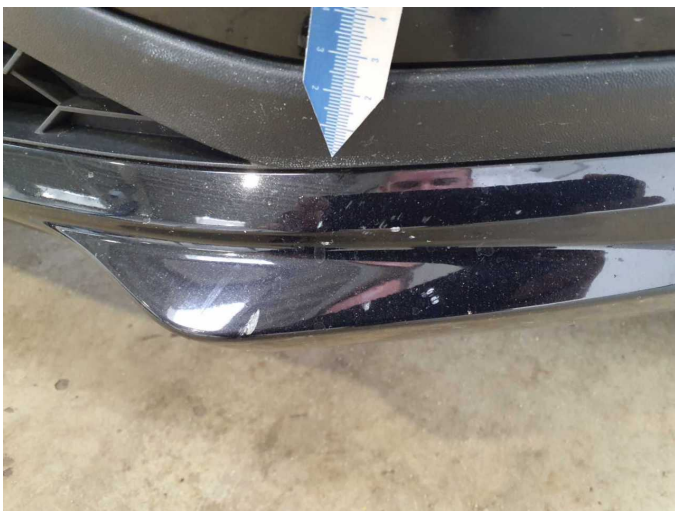
Damage 13: Front bumper: Front bumper - Scratched - Paint
