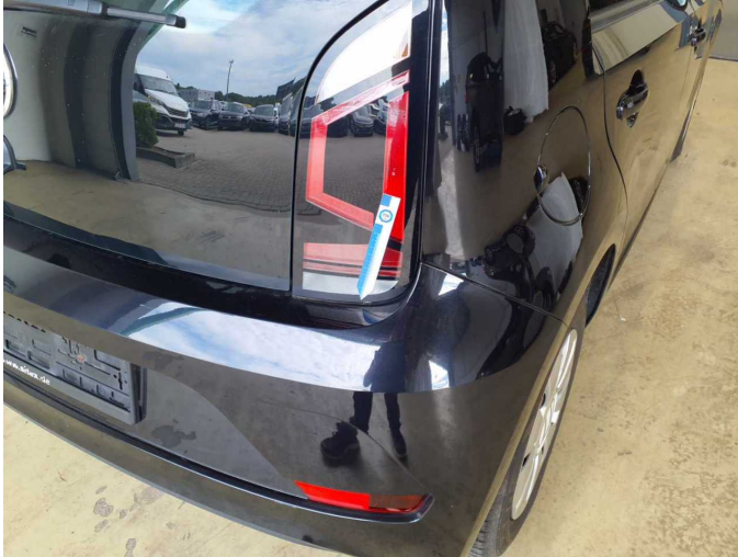
Damage 9: Tail light: Tail lamp - right side - Broken / torn - Replace
