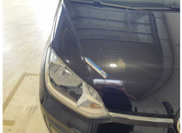
Damage 12: Bonnet: Bonnet - Stone chips - Paint
