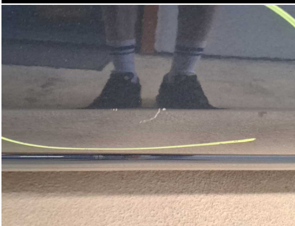
Damage #5: Door - front left side: Door - Scratched - Repair and paint
