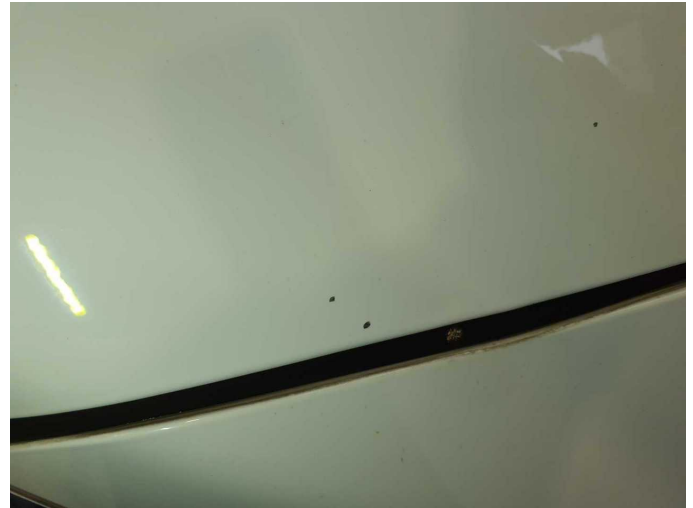
Damage 13: Bonnet: Bonnet - Stone chips - Paint
