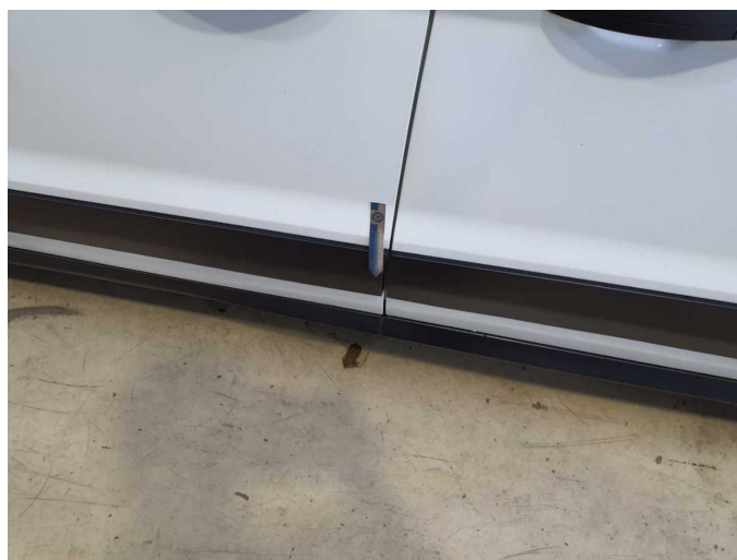
Damage 11: Door - front left side: Brightware - lower - Scratch(es) - Smart repair
