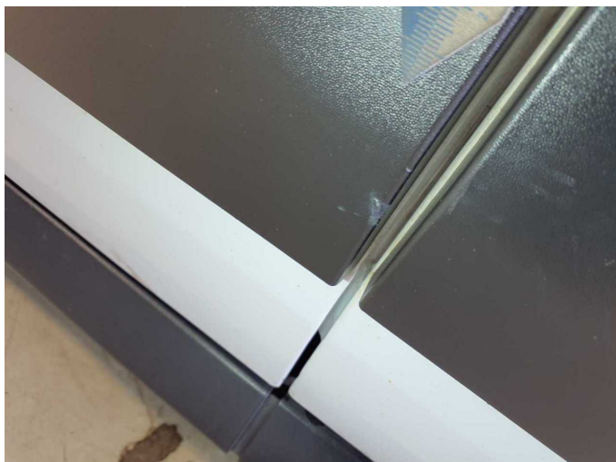
Damage 11: Door - front left side: Brightware - lower - Scratch(es) - Smart repair
