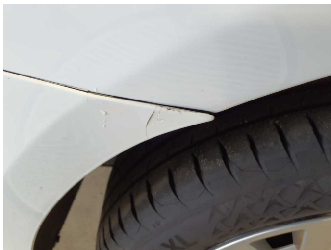
Damage 12: Rear bumper: Bumper - rear right side - Dent / paintcoat damage - Replace
