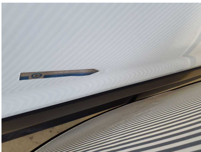
Damage 7: Sliding door, right: Sliding door - Dent / paintcoat damage - Smart repair
