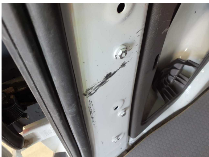
Damage 6: Body: D-pillar - left side - Scratch(es) - Smart repair
