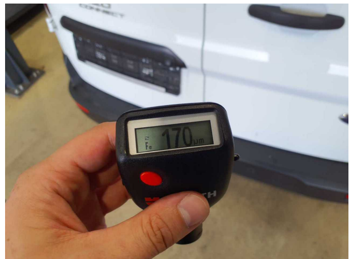
Repainting 1: Boot lid / rear door
