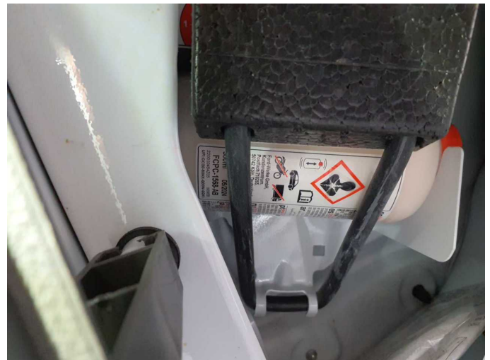
Damage 3: Equipment: Tirefit filler - Expired - Replace
