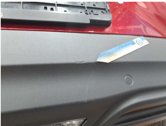
Damage 1: Rear bumper: Rear bumper - Scratch(es) - Loss in value
