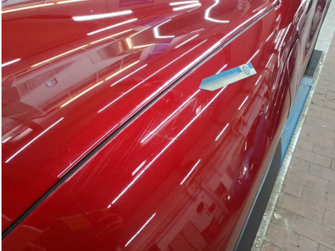
Damage 9: Mudguard - right side: Mudguard - right side - Scratch(es) - Paint
