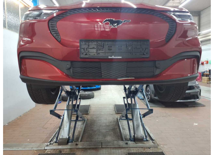
Damage 8: Front bumper: Front bumper (Zierleiste) - Deformed - Replace
