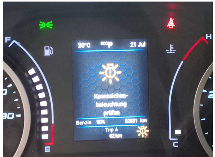
Damage 1: Tail light: License plate lamp - left side - Specify findings - Perform diagnosis
