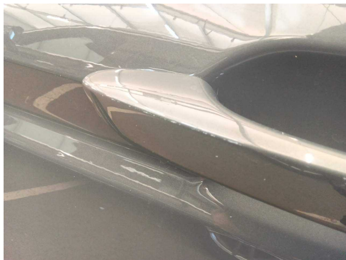
Damage 2: Door - rear left side: Door handle - outside - Scratch(es) - Smart repair
