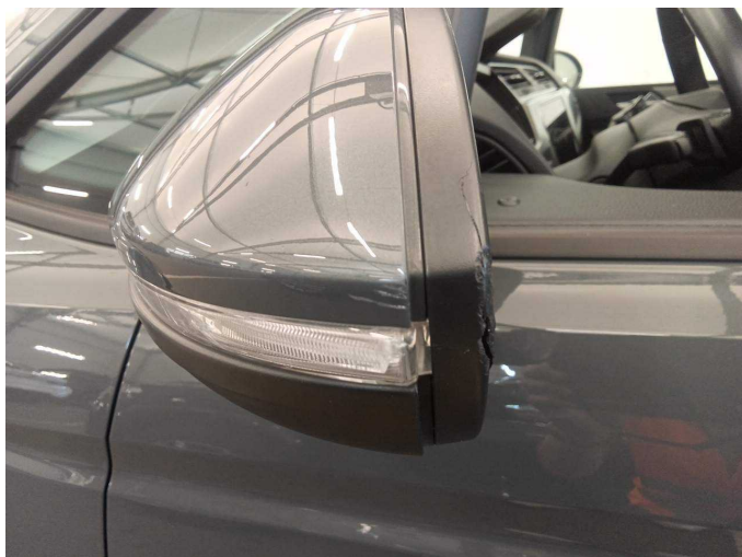
Damage 4: Wing mirror - left side: Chassis - Broken / torn - Replace
