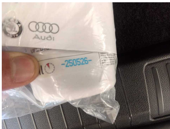
Damage 1: Equipment: Tirefit filler - Expired - Replace
