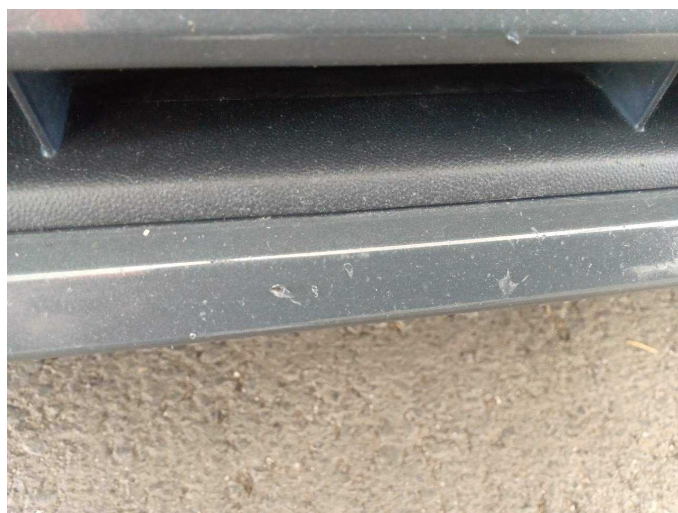
Damage 9: Front bumper: Front bumper (Sandstrahleffekt) - Stone chips - Paint
