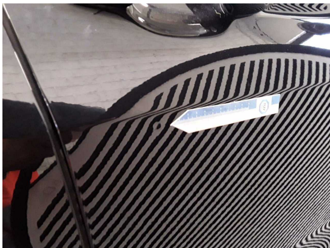
Damage 2: Door - front right side: Door - dent(s) - Smooth repair work
