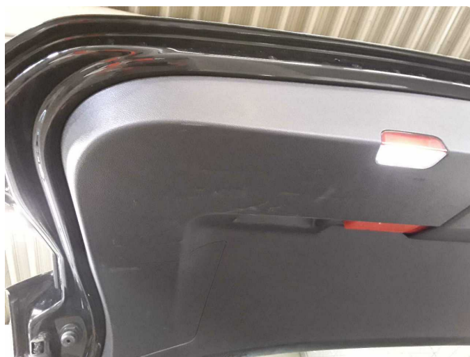
Wear and tear 3: Boot lid / rear door: Trim - standard - lower - Scratched - No deduction
