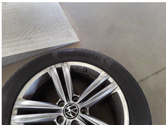
Damage 1: Wheel / tyres: Valve (Reifen HR) - Missing - Replace
