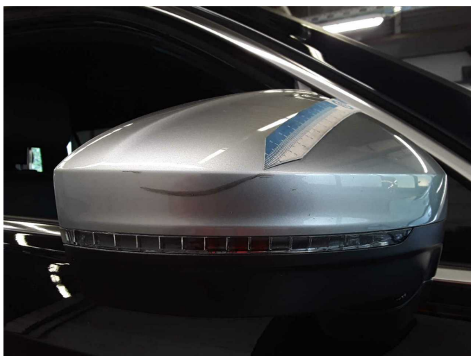
Wear and tear 2: Wing mirror - right side: Mirror housing - Abrasion - No deduction
