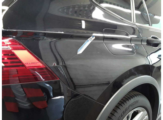
Damage 7: Side panel - rear right side: Side panel - Scratch(es) - Paint
