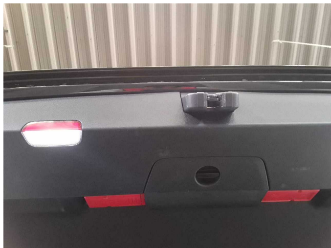
Wear and tear 3: Boot lid / rear door: Trim - standard - lower - Scratched - No deduction
