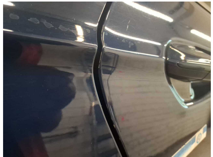
Wear and tear 4: Door - rear right side: Door edge - Scratch(es) - No deduction
