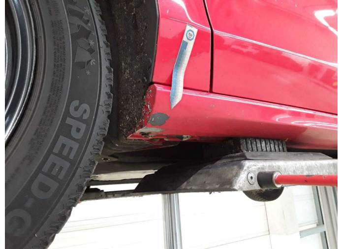
Damage 3: Sill - left side: Trim - Scratched - Smart repair
