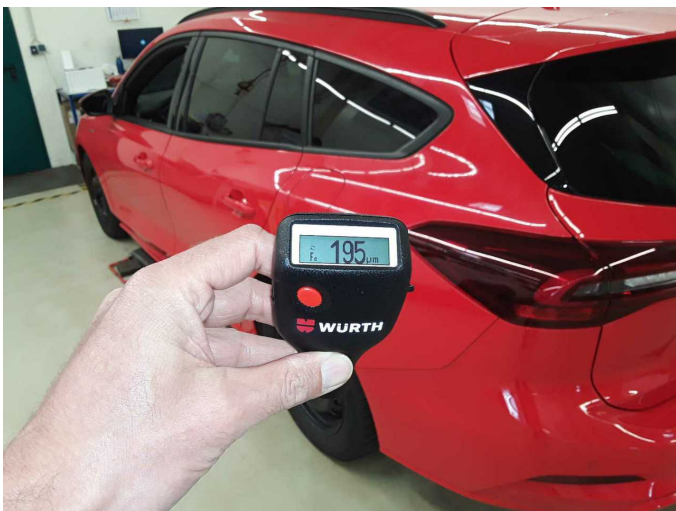
Side panel - rear left side: 195 µm
