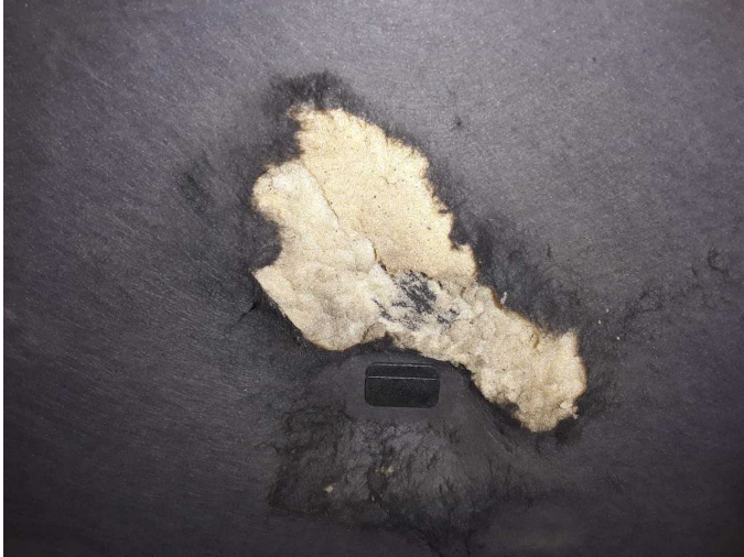
Damage 2: Bonnet: Insulation lining (Marderschaden) - Damage caused by marten / rodent - Replace
