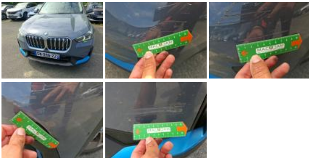
Bumper grille, Broken, Replace
