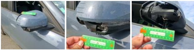
Side repeater R, Missing, Replace
