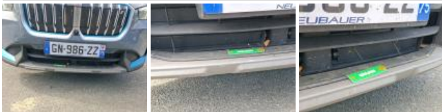
Bumper moulding FL, Broken, Replace
