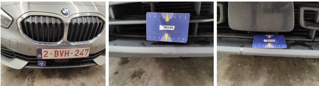
Bumper Front / Trim Left / Replace-scratch
