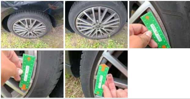
Tyre RR, Tear, Replace
