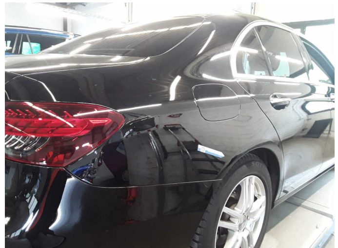
Damage 1: Side panel - rear right side: Side panel - Dent / paintcoat damage - Repair and paint
