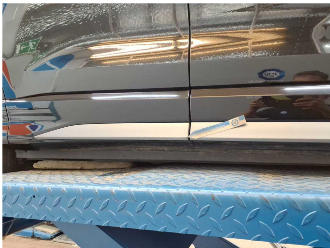
Damage 1: Door - rear right side: Brightware - lower - Scratch(es) - Loss in value
