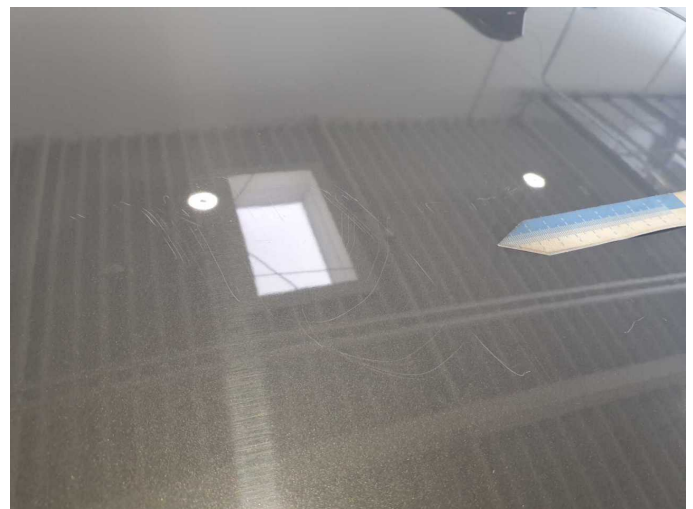
Damage 7: Roof: Roof - Scratch(es) - Paint
