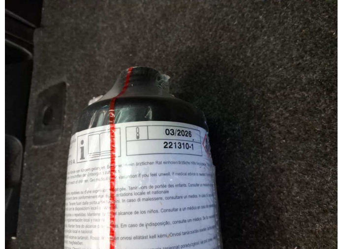
Damage 1: Equipment: Tirefit filler - Expired - Replace
