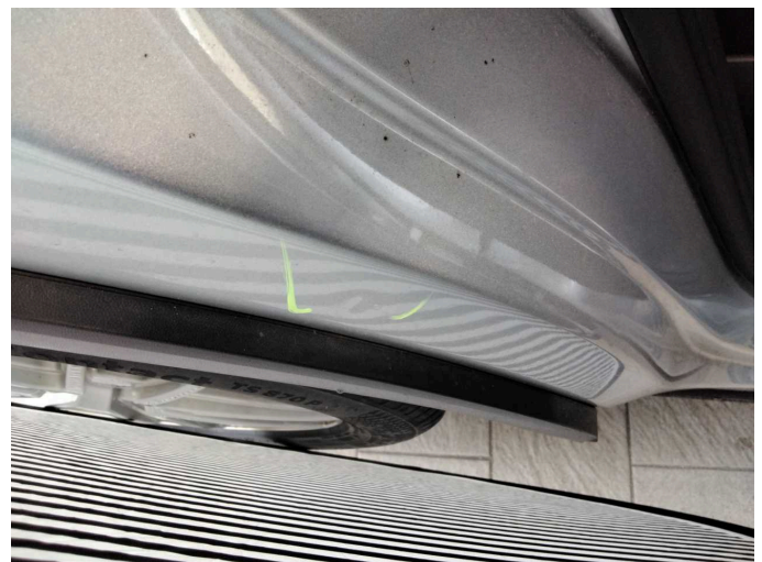
Damage 3: Body: C-pillar - right side - dent(s) - Smart repair
