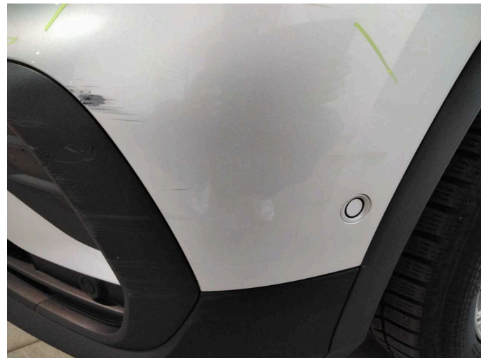
Damage 8: Front bumper: Front bumper - Scratch(es) - Paint
