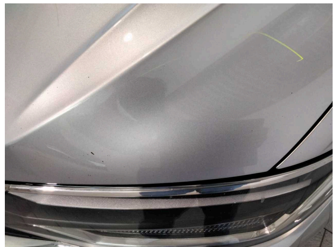
Damage 9: Bonnet: Bonnet - Stone chips - Paint
