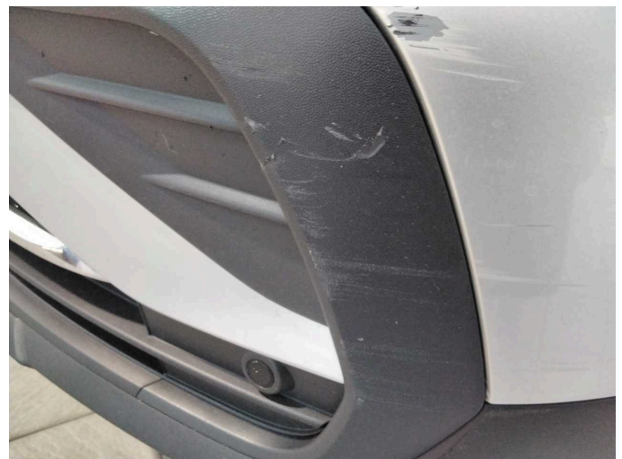
Damage 5: Front bumper: Front bumper (Unterteil) - Scratch(es) - Smart repair
