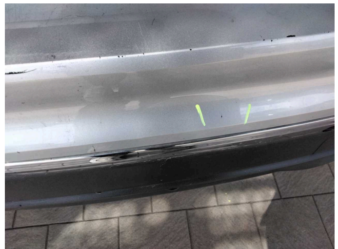
Damage 6: Rear bumper: Rear bumper - Scratch(es) - Paint
