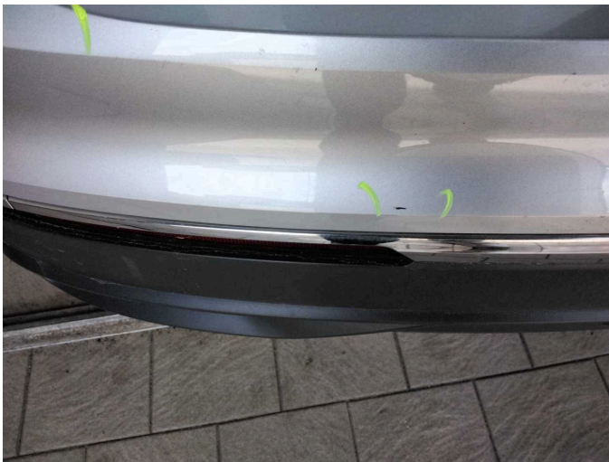
Damage 6: Rear bumper: Rear bumper - Scratch(es) - Paint
