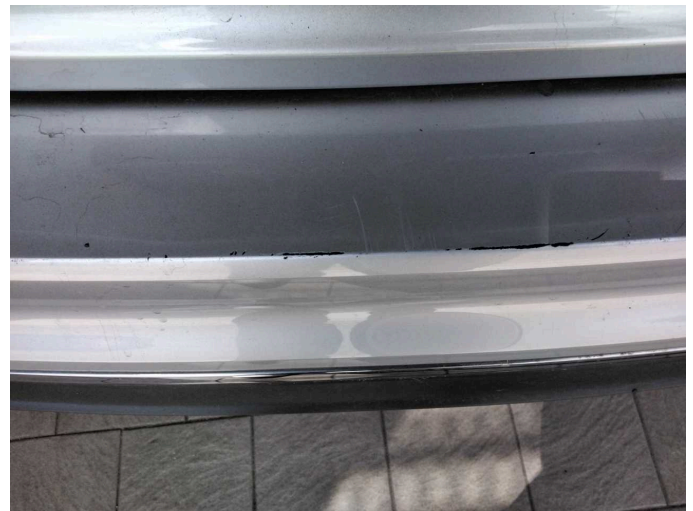
Damage 6: Rear bumper: Rear bumper - Scratch(es) - Paint
