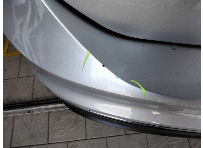
Damage 6: Rear bumper: Rear bumper - Scratch(es) - Paint
