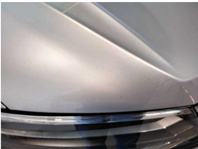
Damage 9: Bonnet: Bonnet - Stone chips - Paint
