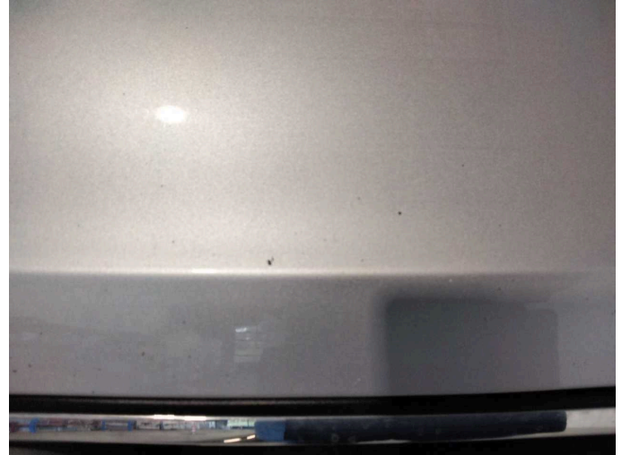
Damage 9: Bonnet: Bonnet - Stone chips - Paint
