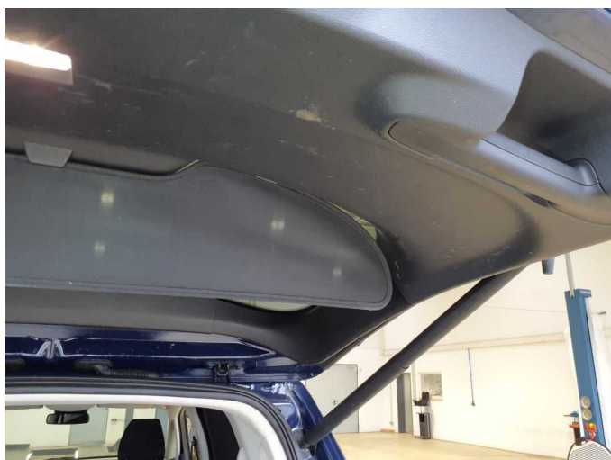
Damage 1: Trim / covers: Trim / covers - Missing - Replace
