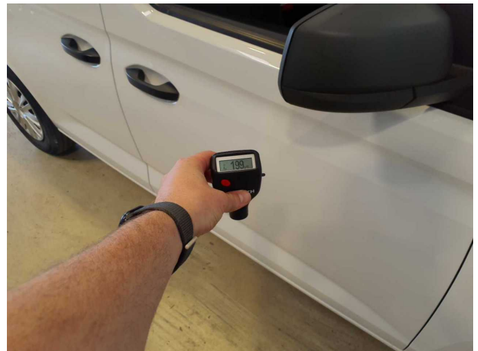
Repainting 2: Door - front right side
