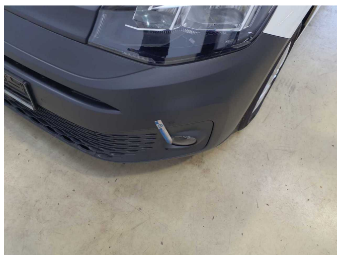
Damage 4: Fog lamp: Fog lamp - front left side - Broken / torn - Replace
