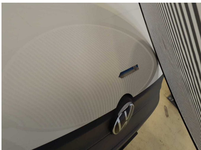
Damage 5: Bonnet: Bonnet - Dent / paintcoat damage - Smart repair
