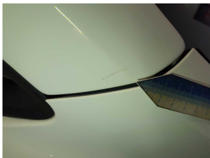
Damage 2: Body: A-pillar - right side - Scratch(es) - Smart repair
