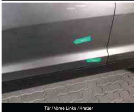
Tür / Vorne Links / Kratzer
