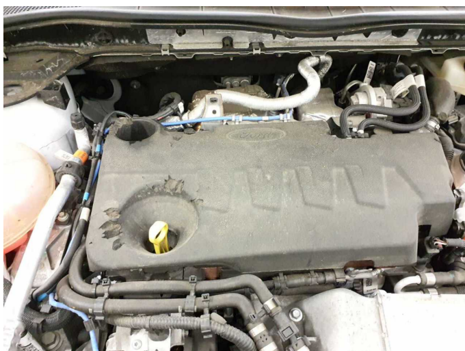
Damage 2: Engine: Engine cowling - Broken / torn - Replace
