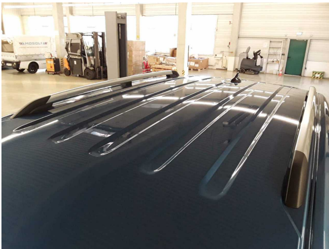
Damage 2: Roof: Roof - dent(s) - Smart repair
