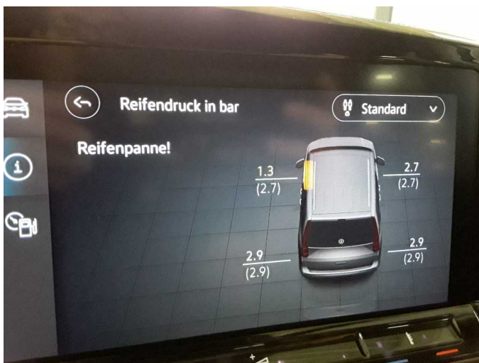
Damage 3: Wheel / tyres: Tyre - front left side - Leaking - Replace
