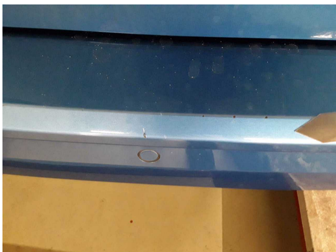
Damage 4: Rear bumper: Bumper with Parktronic - Scratch(es) - Paint
