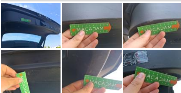
Boot lid covering R, Scratch(es), Replace
