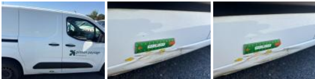
Door trim FR, Deformed / Strained, Replace
