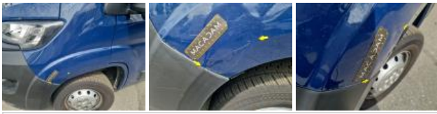
Side repeater L, Broken, Replace
