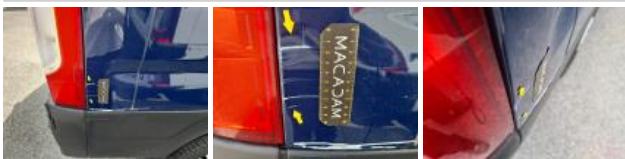
Rear light L, Broken, Replace
