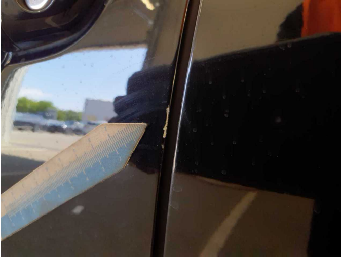
Damage 1: Door - front left side: Door - Dent / paintcoat damage - Smart repair
