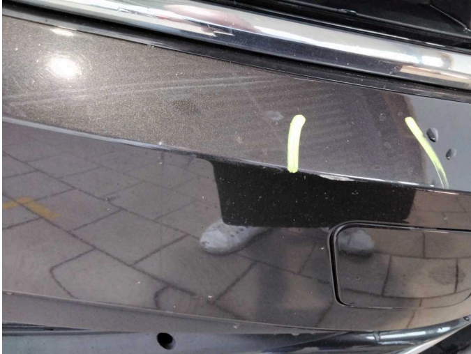
Damage 12: Front bumper: Front bumper - Scratch(es) - Paint
