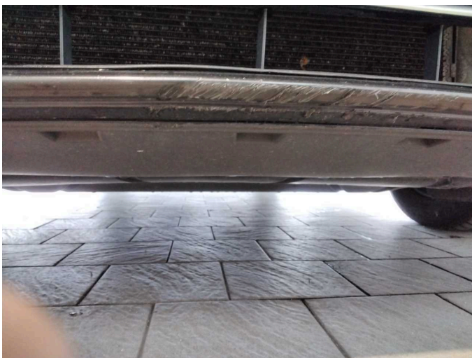
Damage 12: Front bumper: Front bumper - Scratch(es) - Paint
