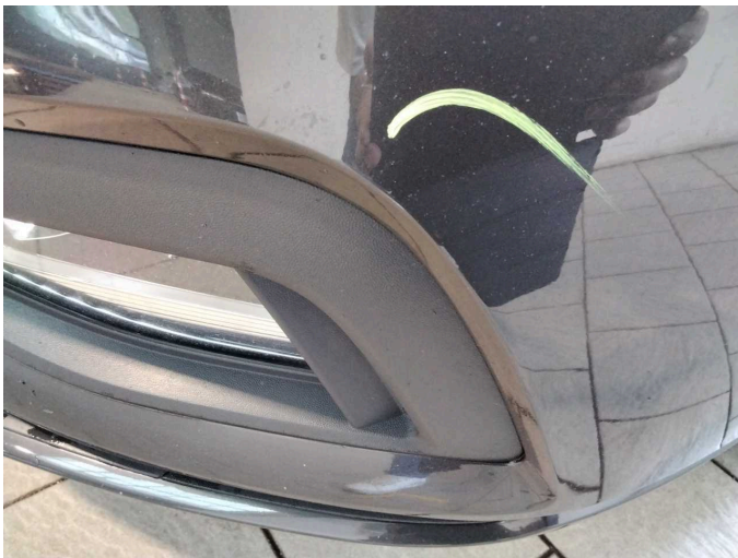
Damage 12: Front bumper: Front bumper - Scratch(es) - Paint
