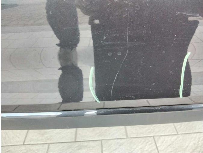
Damage 11: Rear bumper: Rear bumper - Scratch(es) - Paint
