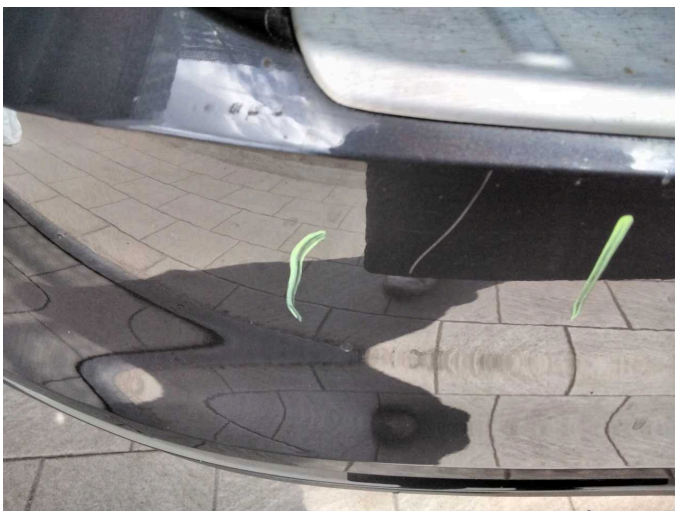
Damage 11: Rear bumper: Rear bumper - Scratch(es) - Paint
