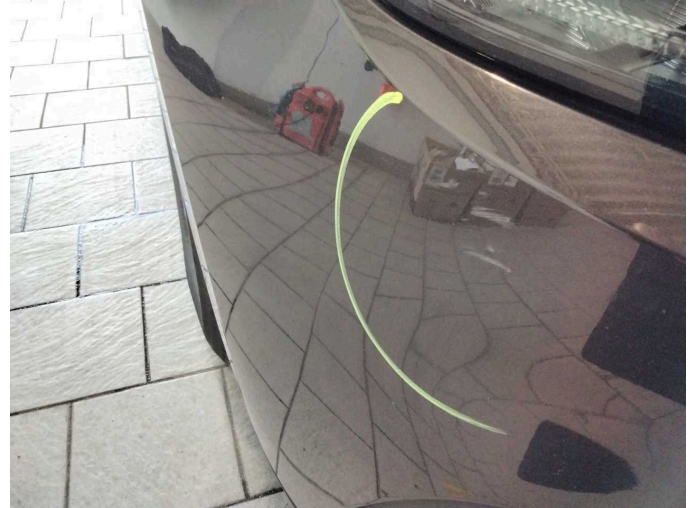
Damage 12: Front bumper: Front bumper - Scratch(es) - Paint
