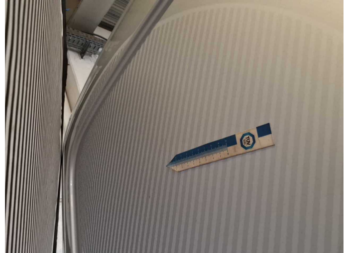
Damage 4: Boot lid / rear door: Rear door - left side - dent(s) - Smooth repair work
